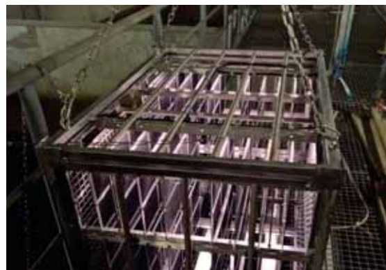
Fig. 4. MOL ® LIK catalyst module (Capacity: up to 2000 m 3 /h water)
